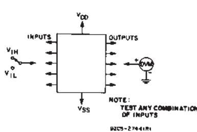
Fig. 14 — Input voltage test circuits.
