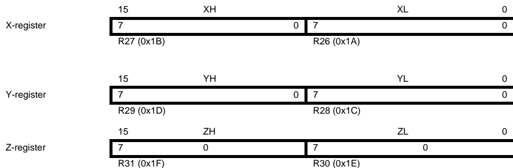
Figure 5. The X-, Y-, and Z-registers
